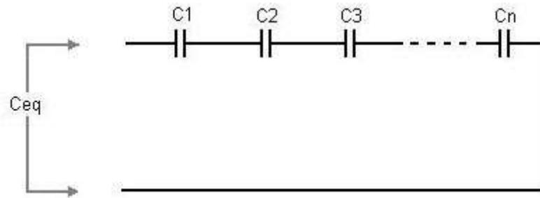
$$\frac{1}{C} = \frac{1}{C_1} + \frac{1}{C_2} + \frac{1}{C_3} + \frac{1}{C_4} + \dots + \frac{1}{C_n}$$
