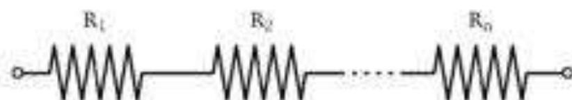
$$R_t = R_1 + R_2 + R_3 + \dots + R_n$$
