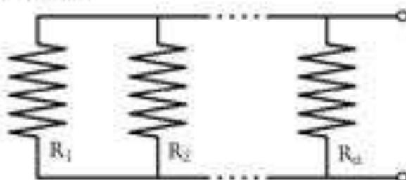
$$\frac{1}{R_t} = \frac{1}{R_1} + \frac{1}{R_2} + \dots + \frac{1}{R_n}$$
