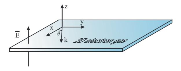
on the surface of a solid or in heterostructures the inversion symmetry is broken and SOC can lift the degeneracy of the states
