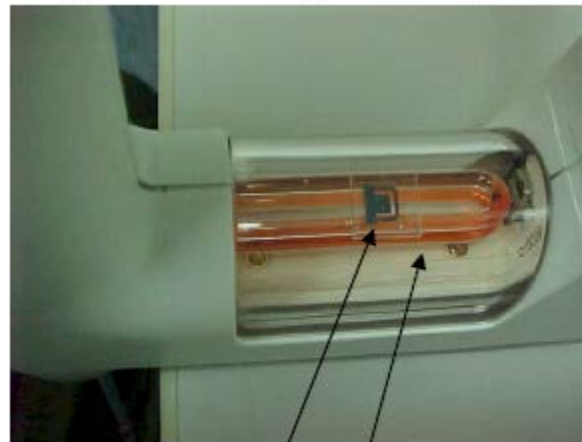
Figure 2. Silicon microtube sensor chip on top of a conventional glass tube sensor.
